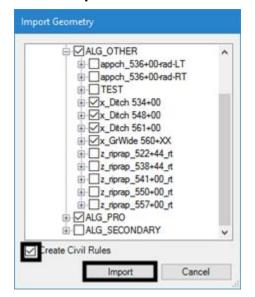
The alignments are imported. The centerline for the roadway is in the middle part of the terrain model and the other alignments are scattered throughout along the centerline.
