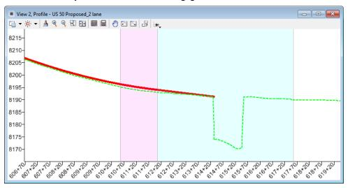
21. In the Profile View (*View 2* in this example), Select the vertical alignment element and **Open Element Information**.
