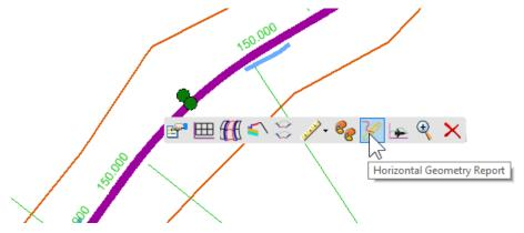
The report can be used to verify the import was successful. Also, a review of the start and end stations shows that the centerline length is about 3.7 miles long. This is fine for the alignment but we will want to be watchful after the corridor is imported to see if it performs well when editing and is stable. Generally, we will want to keep corridor lengths to less than 2 miles for best computer performance. We will keep this in mind when we get to the next section.
