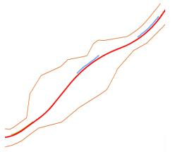
14. At this point, notice that there appears to be duplicate elements shown in the view. This is because the 3D model created by OpenRoads is automatically referenced to the 2D model. In **Reference Manager**, turn off the display of **Default 3D** for better clarity in the view.
