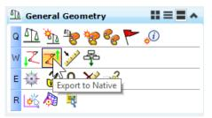
4. When the export command starts, pick the alignments to be exported. The active vertical alignment for the alignment is also exported.
