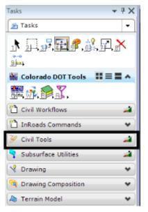
5. Under the *Civil Tools* task, expand the Terrain Model tasks.
